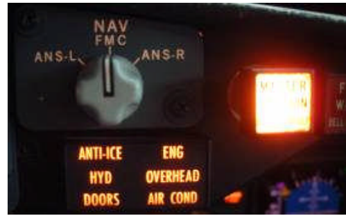
Master Caution and System Annunciator lights, left and right.
