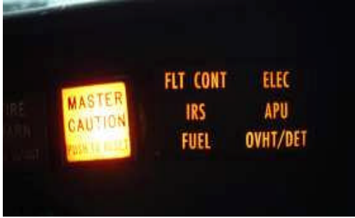
Master Caution and System Annunciator lights, left and right.
