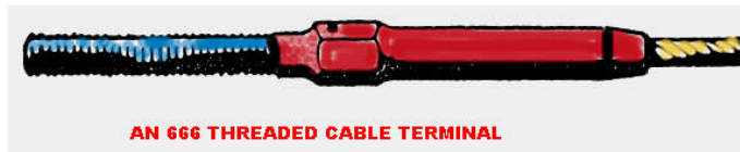
Şekil 5.19: AN 666 threaded cable terminal
