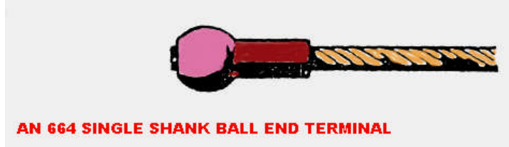
Şekil 5.17: AN 664 single shank ball end terminal
