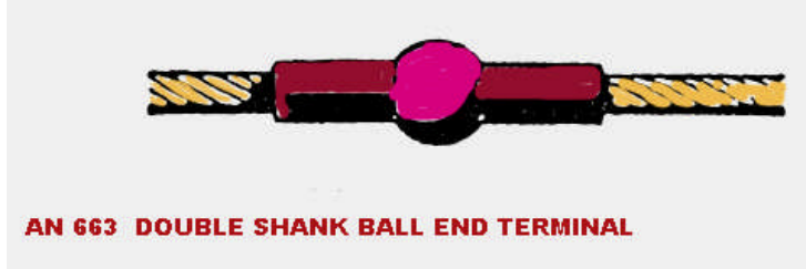
Şekil 5.16: AN 663 double shank ball end terminal
