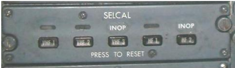
Resim 7.1: SELCAL kokpit paneli
