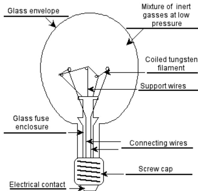
Figure 5.6: A light bulb's structure
