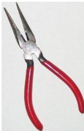
**Figure 3.13: Needle nose pliers**
