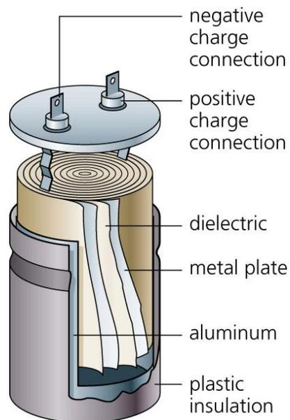
**Figure 5.9: Structure of an electrolytic capacitor.**
