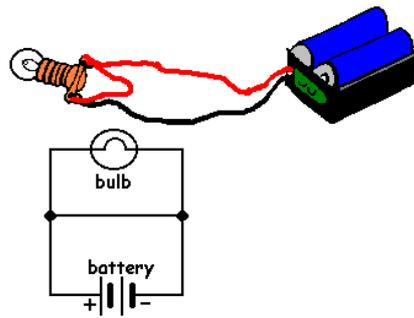
Figure 5.28: Short circuit
