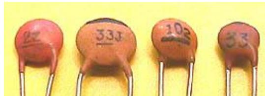
**Figure 5.8: ceramic capacitors**
