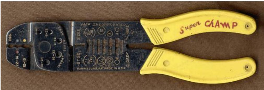
**Figure 3.15: Electrical wire stripping and terminal crimping pliers**
