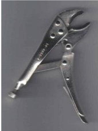
**Figure 3.17: Lock jaw pliers, also called vise grip or "mole grips".**
