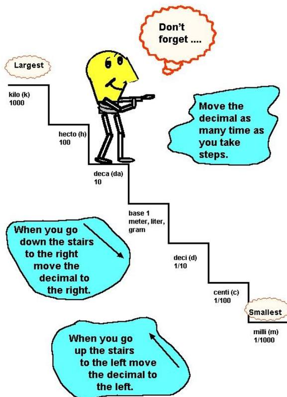
Figure 1.3: Learning main units using the metric staircase
