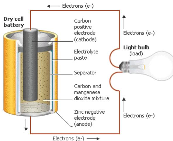
Figure 5.4: Dry cell chemical structure
