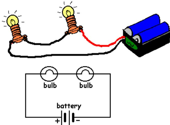
Figure 5.30: Series circuit
