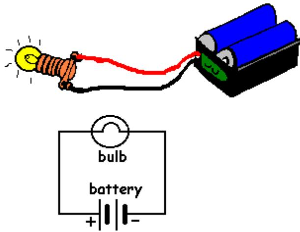
Figure 5.26 Simple circuit
