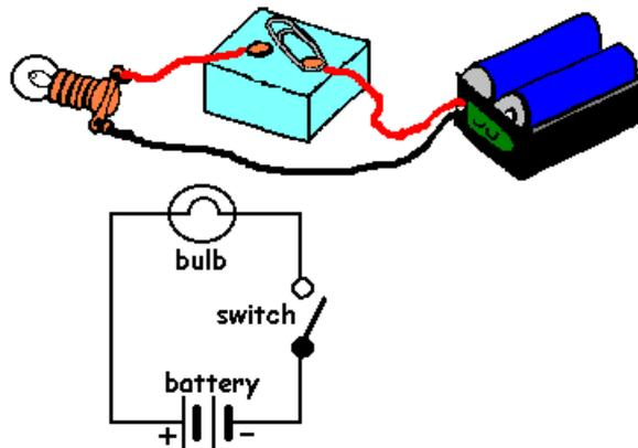
Figure 5.29: Switched circuit
