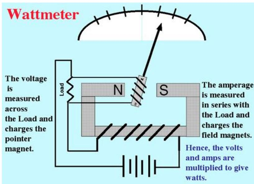
Figure 6.8: Working principle of a wattmeter
