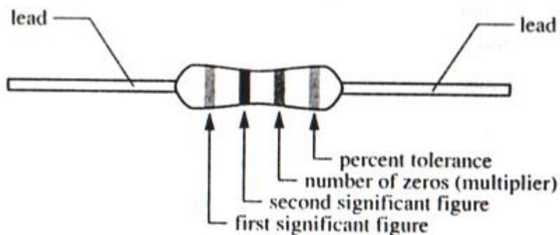
**Figure 5.2: Resistor color coding**
