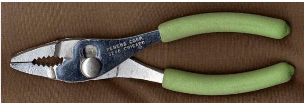
**Figure 3.12: Slip joint pliers**
