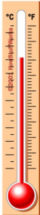
**Figure 1.13: A celcius and fahrenheit scaled thermometer**
