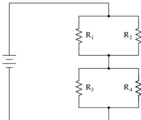
**Figure 5.32: Series-parallel circuit**
