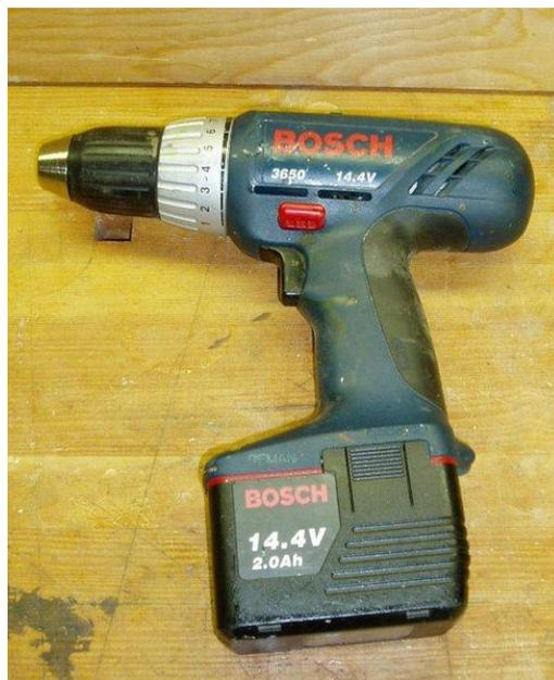
**Figure 3.20: A cordless drill with clutch**
