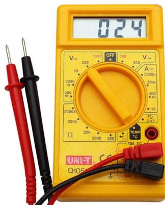
**Figure 6.4: A multimeter**
