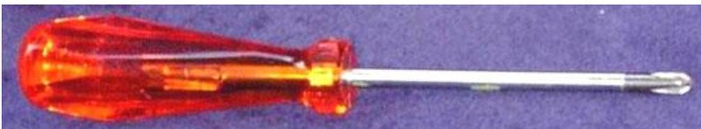
Figure 3.3: a basic phillips screwdriver (star tipped)
