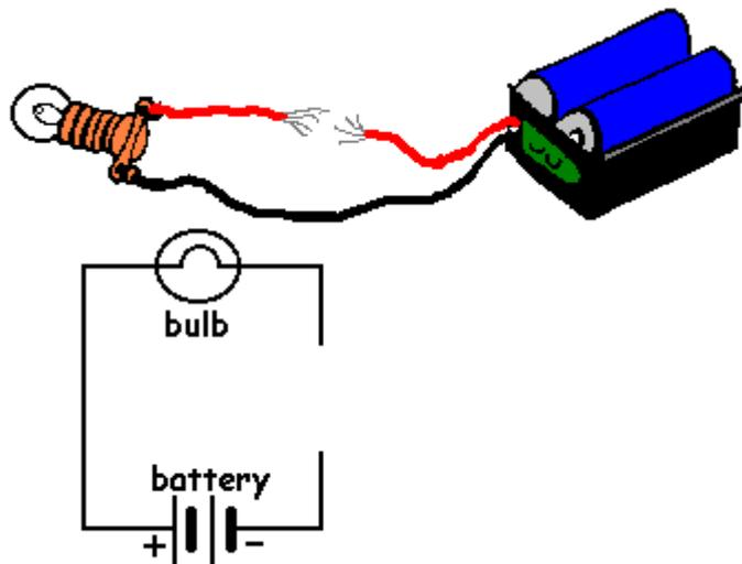
Figure 5.27: Open circuit
