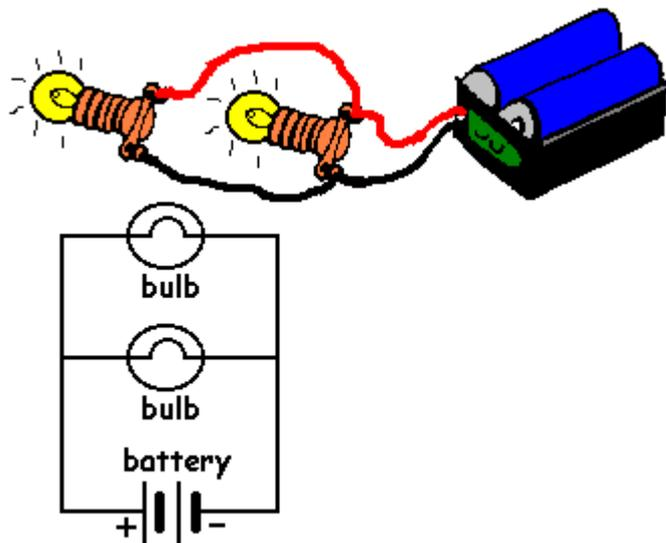
Figure 5.31 Parallel circuit
