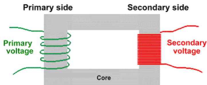
**Figure 5.22: Transformer coils**
